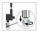
Inserting the filter
